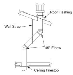
Figure 19 - Offset with Wall Strap and 45° Elbows
